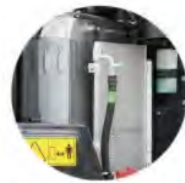
03 Water tank & radiator
