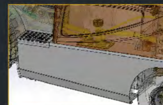
Side mounted welded oil tank
