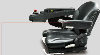
Grammer full suspension seat is optional for more comfortable driving. The multifunctional armrest integrates fingertip switch, direction switch, steering switch, PES gear, horn button, emergency power-off switch, etc., to realize convenient operation and precise control of electromagnetic proportion.
