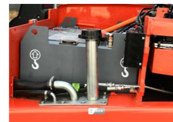
The hydraulic oil tank is located on the left side for easy filling and checking.
