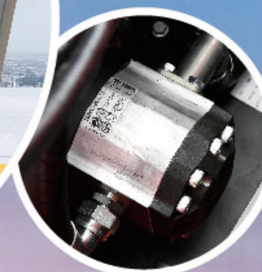
A new generation design of the hidden rubber hose pulley block of the mast, wide view ahead
