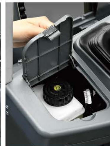
Brake fluid within reach, easy to check and refill
