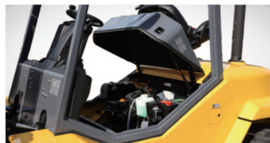
High angle hood open for easy maintenance
