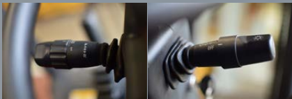
Standard distribution fluid reversing handle + steering, lamp combination handle Improve ease of operation
