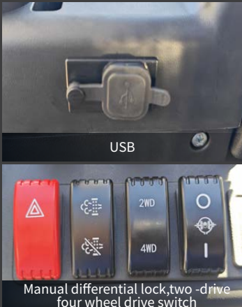
Manual differential lock,two -drive four wheel drive switch
