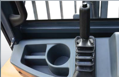
Ratchet type hand brake, reliable movement, small operating force
