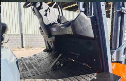
Tilt the cylinder down to improve legroom
